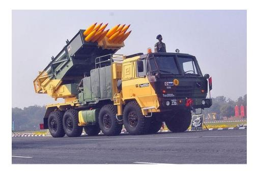
Pinaka is a multi-barrel rocket launcher developed indigenously for the Indian Army and produced in India by involving Public Sector and Private Sector Defence Industries. The multi-barrel launcher system is mounted on the highly rugged BEML truck, much acclaimed for its off-road mobility and would provide the Indian Army with vital manoeuvrability on the battlefield.
