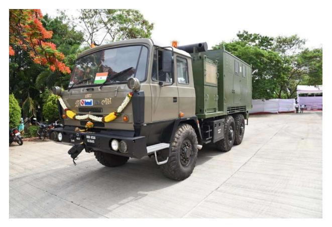
Mechanical Minefield Marking Equipment MK-II developed by R&DE (Engineers) would greatly benefit Indian army to mark/fence minefields. The MK II is designed for marking the mine fields at faster rate, semi-automatically with minimal human intervention.
