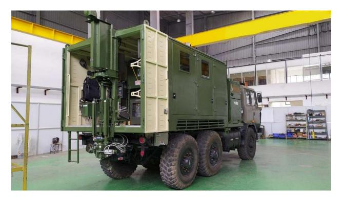
MMME Mk-II system is designed to operate in plains of Punjab, as well as semi-desert & desert of Rajasthan, in all weather conditions. The system can store 500 numbers of pickets and polypropylene rope of 15 km in length.
