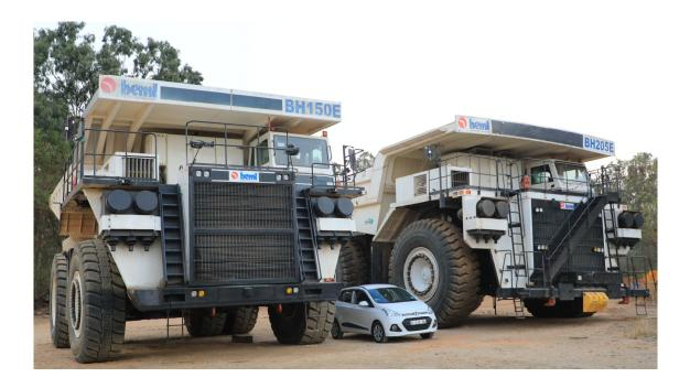
These trucks have eco-friendly emissions certificate engines with electronic fuel management system to deliver maximum power. Its wide body design-higher value metric capacity and low body weight ensures high stability and productivity. A state-of-the-art AC drive system have been engineered to provide exceptional road performance with reduced maintenance.
