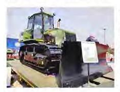
This dozer can be used mainly for clearing debris, making roads areas an exclusive use for Army applications in tough terrains. It can withstand extreme temperature variations from high temperature to minus temperatures.
