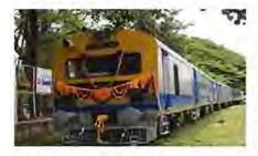
The 3 phase Propulsion system is state-of-the-art system consisting of IGBT based microprocessor controlled 3 phase drive with VVVF (Variable Voltage Variable Frequency) control. The train has regenerative braking system for energy saving, and saves around 30% of energy thus
